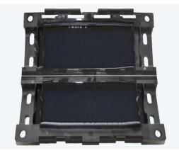
The gel-filled cable joint technique is a new system with special advantages. It is quick and easy to install and reduces the chance of assembly errors. The impact-resistant case is connected by a hinge for easy installation. After closing the cable joint the special gel flows together and ensures a good sealing and insulation of the connection. After installation, the cable joint can be put directly in use. No special tools requiredGood adhesion to metals and plastics
